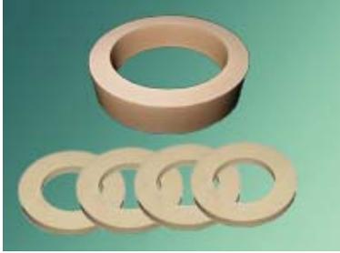
A novel engineering material compounding with PTFE resin and PHB, having good wearing, high temperature and creep-resistance. Applicable environment: temperature  $-200\sim 300^{\circ}\text{C}$ , pressure 25MPa, and 0~14 pH.
